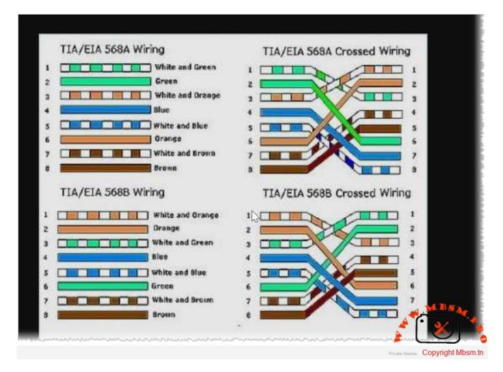
The T568A and T568B standards define the arrangement of wires inside RJ-45 network cables, where each standard specifies a different color order, affecting how cables are connected to devices. The choice between them depends on compatibility with existing infrastructure or personal preference.
