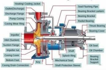
Centrifugal pumps are widely used devices for moving fluids, and they consist of several critical components that work together to perform this function. Here are the main parts of a centrifugal pump:
