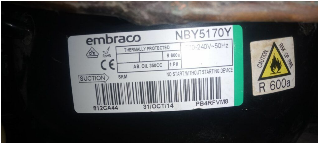
File Pdf: NBY5170Y, Compressor, 1/4 HP, 1ph 220-240V/50Hz, R600a, 15kg, High Back Pressure, HBP, Commercial Refrigeration, Embraco
