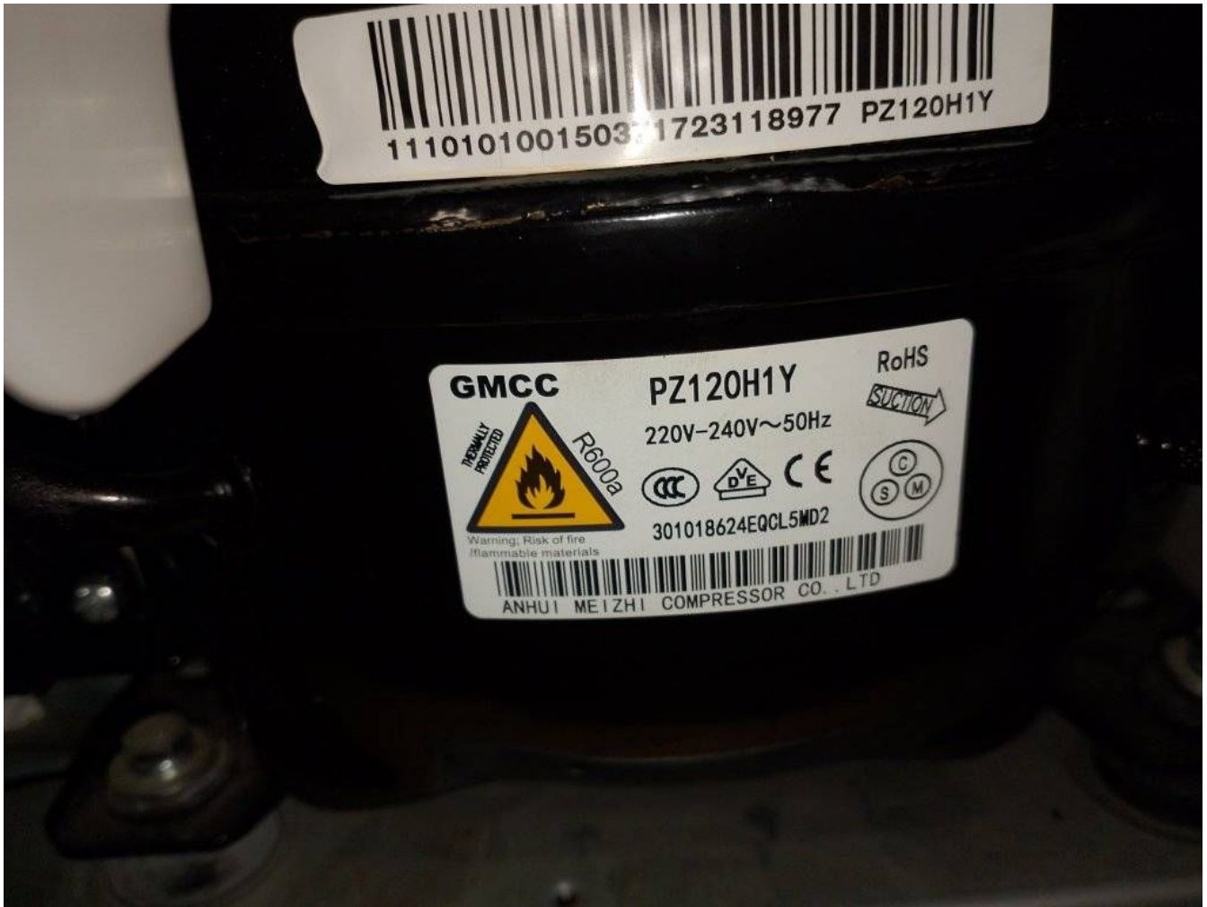
Pdf File, Mbsm.pro, Copressor, GMCC, PZ120H1Y, 1/3 hp, 210 w, lbp, r600a
